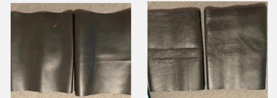
Figure 3 Snagging resistance of the faux leather (Left) and textured faux leather (Right) fabrics
