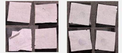
Figure 2 Colorfastness to crocking of the faux leather (Left) and textured faux leather (Right) fabrics; dry test (top) and wet test (bottom)
