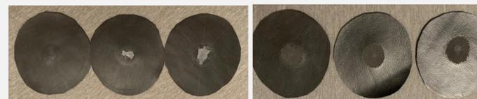
Figure 1 Flat abrasion resistance of the faux leather (Left) and textured faux leather (Right) fabrics: Surface change after 1000, 2000, and 3000 cycles respectively
