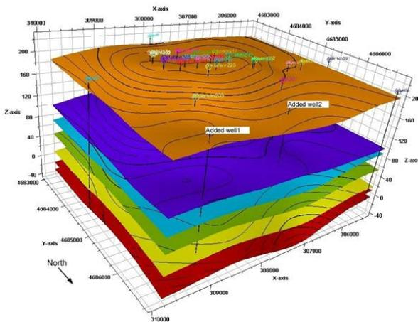
Figure 7. The second model three-dimensional model outlining the two new synthetic wells as well as the seven unit horizons: Ancell, Trempealeau, Franconia, Ironton-Galesville, Eau Claire Proviso A and B, Eau Claire Proviso C “Lightsville” (top), and (bottom)
