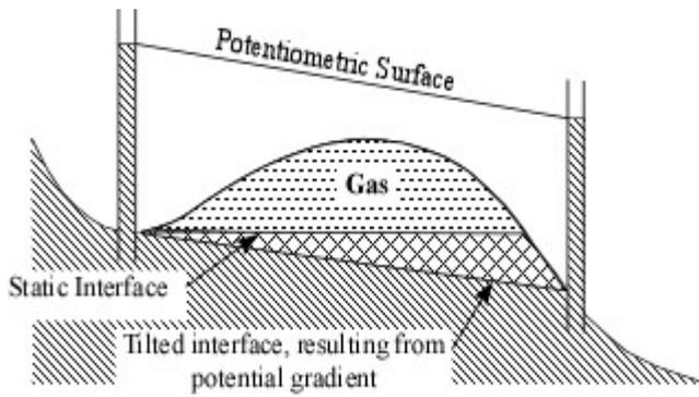
Figure 2. Schematic diagram of the tilted gas-water interface at Pecatonica (from [11])
