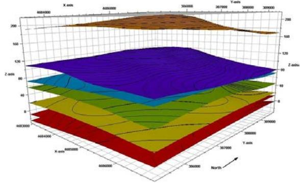
Figure 6. Initial 3-D model with geologic horizons interpreted by Petrel: Ancell, Trempealeau, Franconia, Ironton-Galesville, Eau Claire Proviso A and B, Eau Claire Proviso C “Lightsville” (top), and (bottom)
