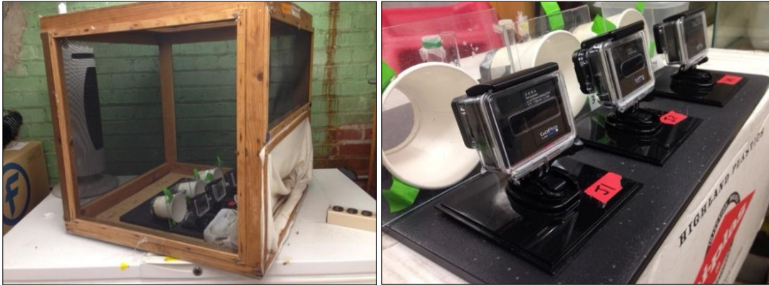
Figure 2.1. Materials and Methods of Behavioral Assays. Mating trials in a 60 cm 3 cage containing a colony of mosquitoes, a tower fan and a pair of socks to stimulate mating behaviors (left). Three mating arenas and 3 cameras secured with hook-and-loop fasteners to a plastic cutting board for ease of transfer to the colony cage (right).
