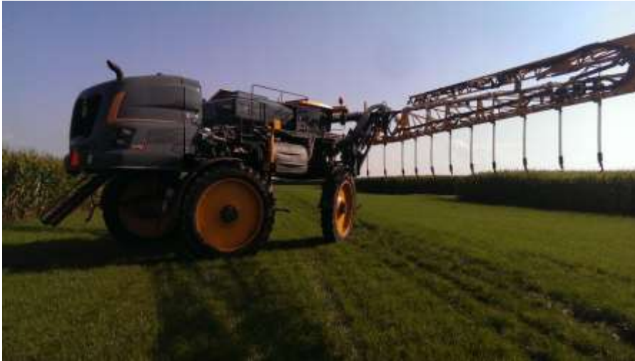
Figure 2. Hagie STS modified with air seeder used to plant cover crops.
