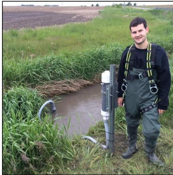
Figure 5. The PVC Stilling well (in the stream) connected by conduit to the onshore PVC Unit. I secured both ends to metal posts.
