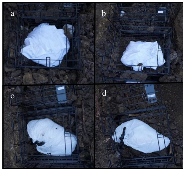
Figure 14. Specimens at 6 inches: a) specimen B in cage 1; b) specimen D in cage 2; c) specimen F in cage 3; d) specimen H in cage 4.
