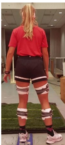
Figure 5. Retroreflective marker placement on the subject.
