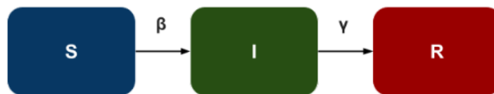
Figure 1: Compartmental model with three classes: S, I, and R. The parameters \beta and \gamma each represent flow rates between classes. In this diagram, \beta is the rate at which the susceptible become infected and \gamma is the rate at which the infected recover.
