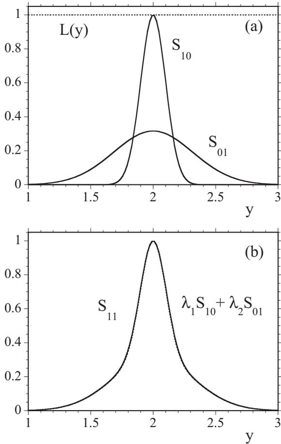
FIG. 1. (a) The shadow functions  $S_{10}(y)$  and  $S_{01}(y)$ , for  $m_s = 0.3$ ,  $m_a = 1$ , and  $D_a = 0.1$  together with the brightness function of the incoming light,  $L(y) = 1$  (dashed line) corresponding to  $\sigma = \infty$ . (b) The shadow pattern obtained from two absorbers  $S_{11}(y)$  together with a best-fit superposition of  $S_{10}(y)$  and  $S_{01}(y)$  shown by the dashed line.
