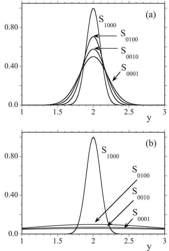
FIG. 3. The four shadow functions  $S_{1000}(y)$ ,  $S_{0100}(y)$ ,  $S_{0010}(y)$ , and  $S_{0001}(y)$  for absorption strength  $m_a=1$ , absorber diameter  $D_a=0.1$ , and incoming light width  $\sigma=\infty$ . The corresponding weight factors of these four modes are displayed in Table I(a) and Table I(b) for 11 arrangements of absorbers. (a) Scattering strength  $m_s=0.1$  and (b) scattering strength  $m_s=1.0$ .
