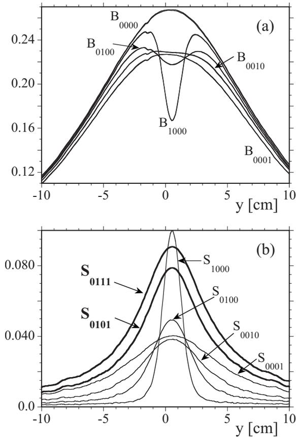
FIG. 5. (a) Experimental brightness functions  $B_{0000}(y)$ ,  $B_{1000}(y)$ ,  $B_{0100}(y)$ ,  $B_{0010}(y)$ , and  $B_{0001}(y)$  for two sets of data. (b) Four experimental shadow calibration functions together with the two- and three-absorber shadows  $S_{0101}(y)$  and  $S_{0111}(y)$ . The corresponding weights for this superposition can be found in Table I(c). The scattering medium was a mixture of 100 ml of 2% milk with 9.2 l of water.
