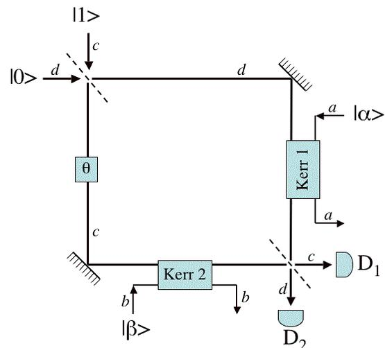
FIG. 1. (Color online) A Mach-Zehnder interferometer, injected with a single photon in the  $c$  mode, with cross-Kerr media placed in each arm. The Kerr media are fed coherent states  $|\alpha\rangle_a$  and  $|\beta\rangle_b$ .  $D_1$  and  $D_2$  are the detectors at output.
