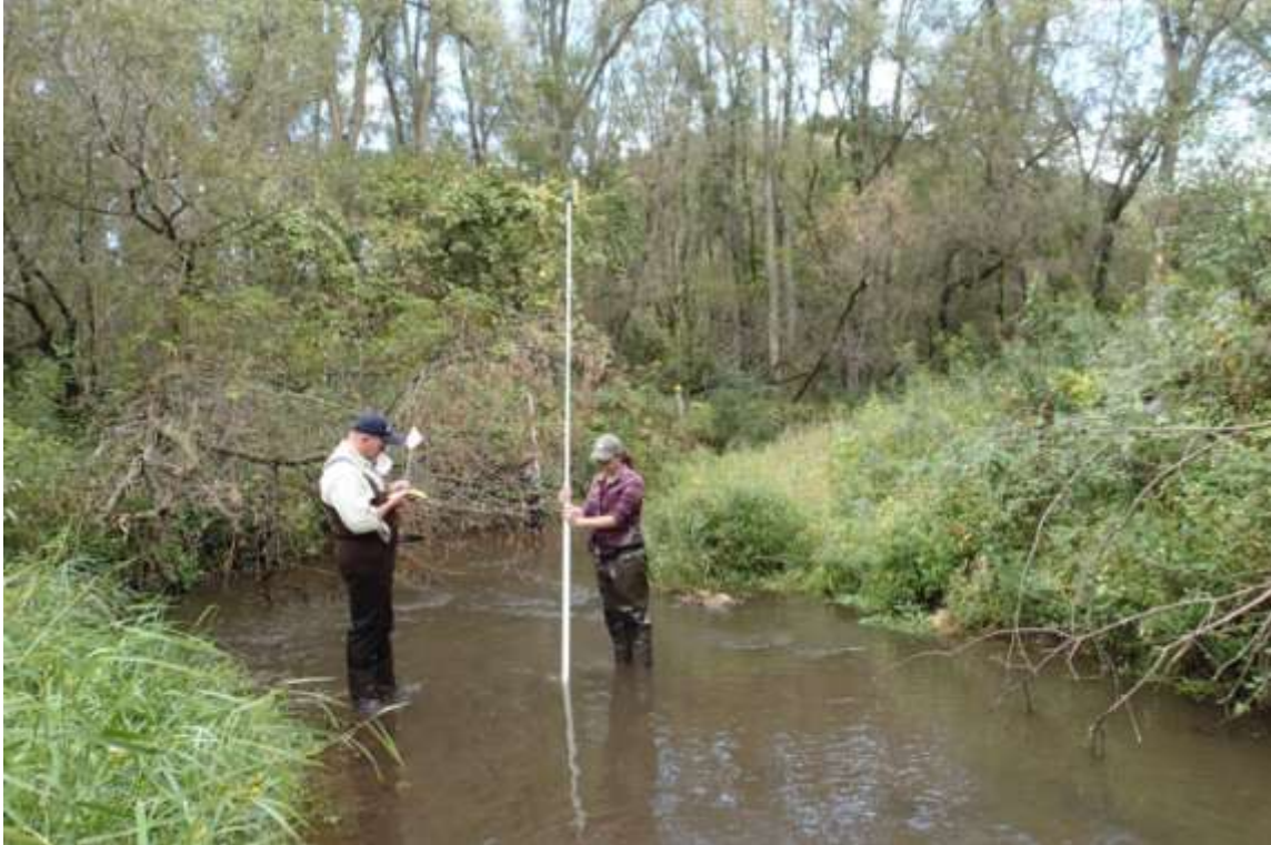
Figure 7- Laserometer HL700 was Attached to the Top of the Stadia Rod that was Raised until it Reached the Laser Station.
