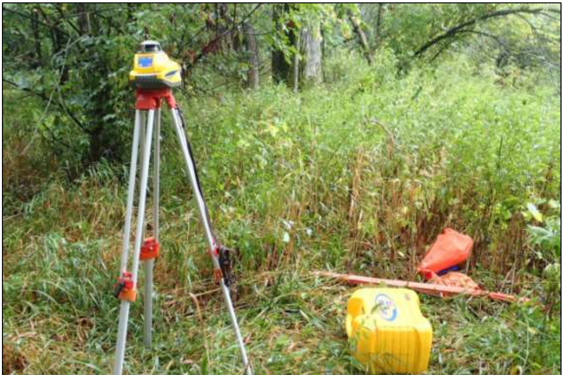
Figure 6- Spectra Precision GL422 Grade Laser Equipment Used to Survey the Streams.
